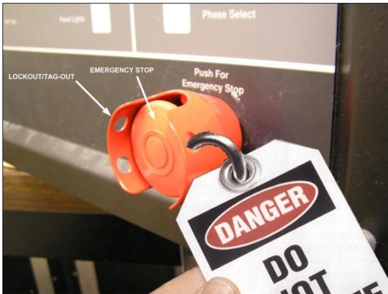
E-stop switch with lockable shroud
